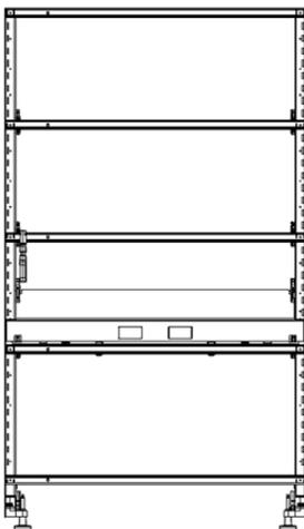
**Basic Frames** do not include the electrical cover kit but may house power which is to be accessed at all locations with a "cut out" tile. The basic frame comes with one wire manager. Basic frames are available for both the 3.5" and 2.75" thick frames. Basic heights available include 24", 29", 37", 44", 51", 57" and 64". The 3.5" thick frame by 24" h includes the mounting hardware to attach to a Planna case where used in a benching application.
