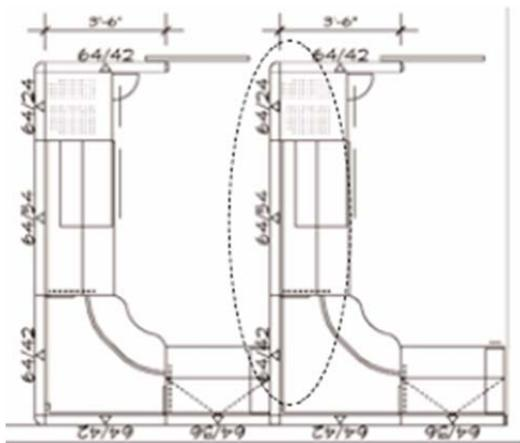
The above image is a correct application of this typical providing sufficient support to the center of the panel from the adjacent workstation.
