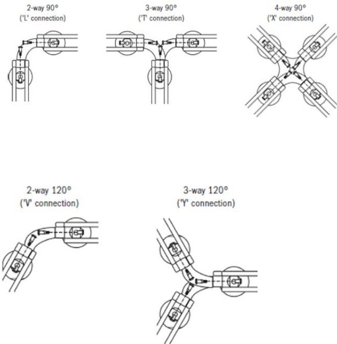
**Inline connectors** are specified to join two frames together which are in alignment. These connectors are specified based on the height of the panels.
