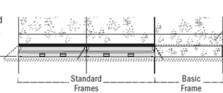
If a basic frame is specified adjacent to a standard frame, a full-height tile must be specified at beltline. In this application, there will be an interruption in the black reveal line.
