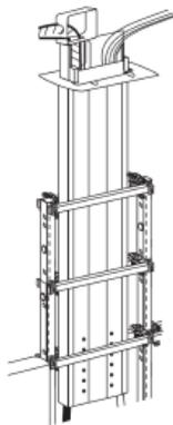
**Power Tracks** are specified for frames 30" wide and wider. This power track mounts at the beltline location of a 3.5" thick
