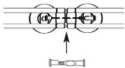
**Off module connections** are specific for frame thickness as well as location where the panel will be mounted to the spine. The off-module panel may be positioned at the end of the panel or in the middle of the panel, with the corresponding bracket. See Inscape System Application Guide.
