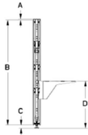
Note: Dimensions 'C' & 'D' measured with frames at lowest glide position. Frame can be raised up to 1.500" depending on configuration and leveling.
