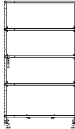
Both types of frames feature glides that provide 1.5" height adjustment allowing air to circulate under panels and throughout the office. Frames are available in 6" increments in widths ranging from 18" wide to 60" wide.
